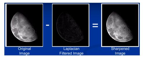
We can apply all these steps using a single mask that is the following (obtained by subtrating the original image to the laplancian filter image):
