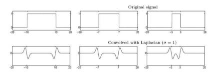
However, our aim is to have a single point between the two ripples. We could increase the  $\sigma$  of the laplancian, but this will end up having a flattened function. So we can multiply the Laplacian by  $\sigma^2$ , after using a trial and error we can find the right value for sigma in order to have a single point rather than having an area.
