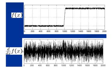
The solution is to smooth the image using the seen filters, in this way the function should be able to spot a single peak rather than detect the noise peaks.
