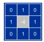
The result of the laplancian filter is not an enhanced image, in fact, we have to subtract this image to the original one to achieve a sharpened image.
