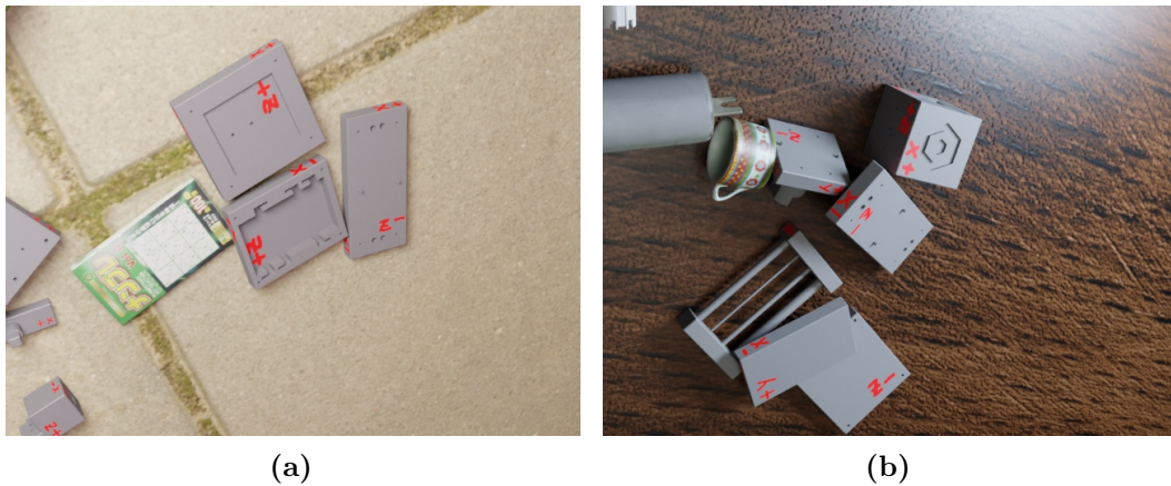
Figure 6.11. In the two figures we can see the examples of industrial textures used in experiment XI. Each object is clearly marked according to industrial convention. This provides a more realistic example, as these markers can be easily replicated during the piece creation process. The solid color used for the object is the default blender color, however, it may be adjusted during the production.
